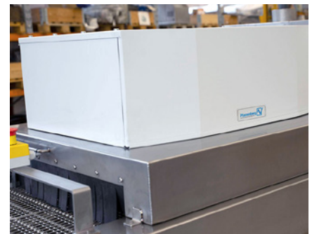
Cooling after cleaning
